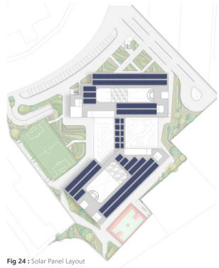
SYSTEM 2 : Azimuth = 135° Tilt = 20° Number of panels = 418 Wattage of one panel = 380W System Size = 158.84 kW Other Parameters entered in PV Watts (same for both systems) : Module Type : Premium Array Type : Fixed (roof mount) System losses : 15% Inverter Efficiency : 96% DC to AC Ratio : 1.2
