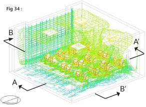
The objective was to move the air breathed out, away from the occupants, before it recirculated back to them. This was achieved by tilting the diffuser air throw slightly. The duct comes from the lower level of the wall, and each diffuser throws the air at a rate of 115 L/s, at a speed of 2.5 m/s. Further, the exhaust vents are placed at the upper level of the opposite wall, so that the return air is drawn out and picked up and exhausted out. This was achieved after multiple iterations.
