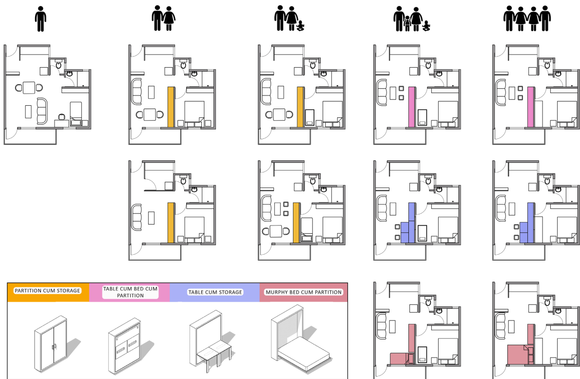
Fig. 17 Possible alterations to interior layouts with change in family structure to increase tenure time
