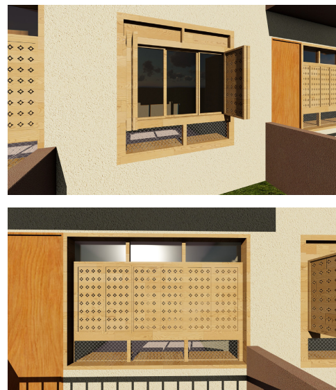
Fig. 32 Vertical shading incorporated as window shutter to avoid additional dead weights
