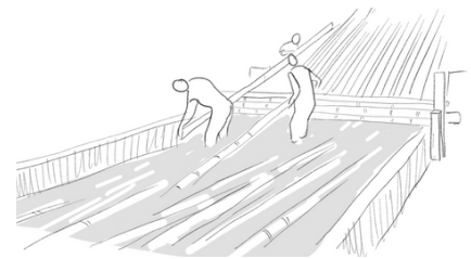
Treatment -Cold soak method where the bamboo is dipped in sol. of boric acid for 7-14 days
