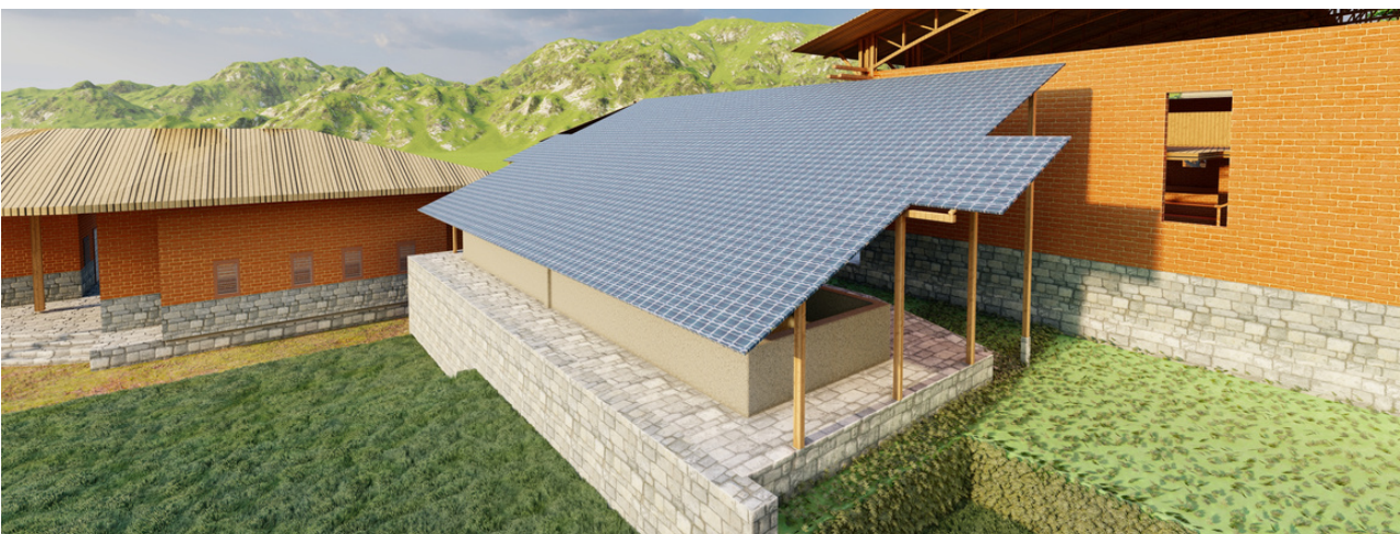
Fig 31: PV Module layout- view
