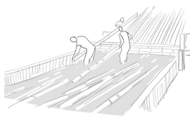
Treatment -Cold soak method where the bamboo is dipped in sol. of boric acid for 7-14 days
