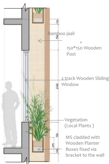
Fig.87 Window detail section :North-Eastern facade
