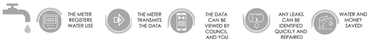
Fig. 11. Process of water metering
