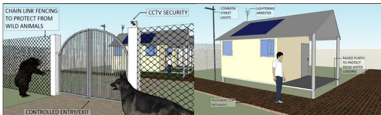
Figure 18: Sketches Illustrating Provisions for making the development Resilient.
