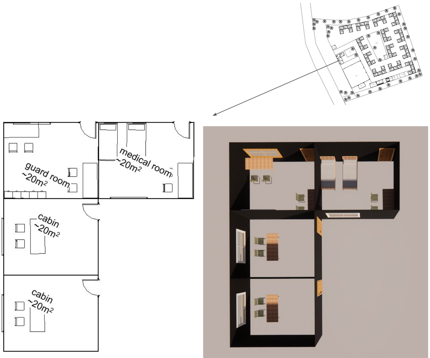
Figure 5. Guard room, medical room and cabins plan
