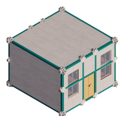
Step 6- Attaching the roof with the structure using main and support beams.
