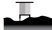
our proposal telescopic plinth stand to adjust acc. base conditions
