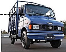
Tata 407 Capacity: 2300 Kg Details: With a dimension size of 9.5ft x 5.5ft x 5.5ft. This is an ideal vehicle light loading..
