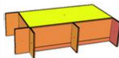
Fig c: Block model with vertical shading. Solar radiation values are : South : 1113 kWh/m 2 East : 1084 kWh/m 2
