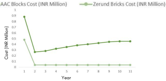
Figure 10.7.c: Life Cycle Costing - Wall Material
