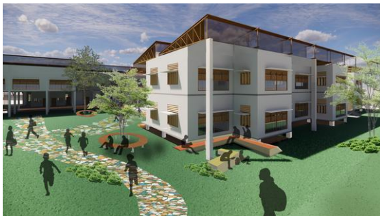
Figure 10.9.m: View of self-shaded spaces due to staggering of the building
