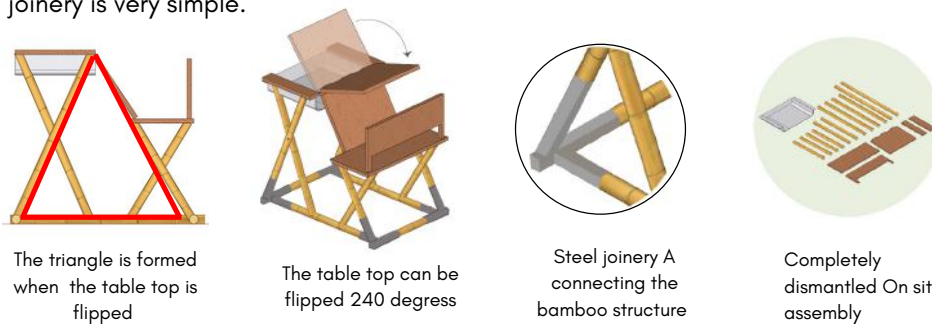
Figure 10.8.k Earthquake shield bench
