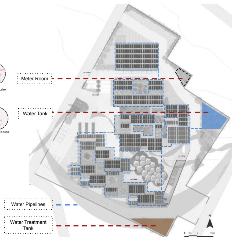
Fig. 5.4.5.2. Rainwater Harvesting Layout
