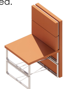
Fig. 5.2.4.4. Convertible Chair with Wooden Panel Placed as Seat & Visible Scissor Mechanism
