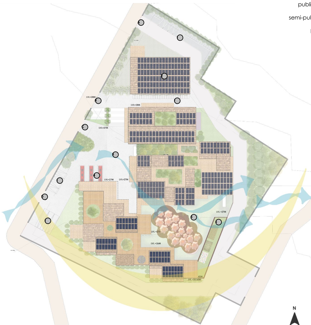
Fig. 5.1.3.3. Modulating the form by staggering it as per the predominant wind-direction and sun-path.
