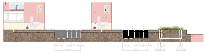
Fig. 5.4.3.2. Schematic Section Recycling Grey & Black Water
