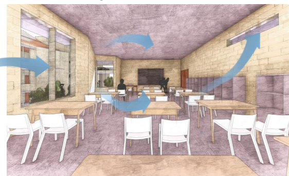
Fig. - cross ventilation in regularly occupied spaces classroom
