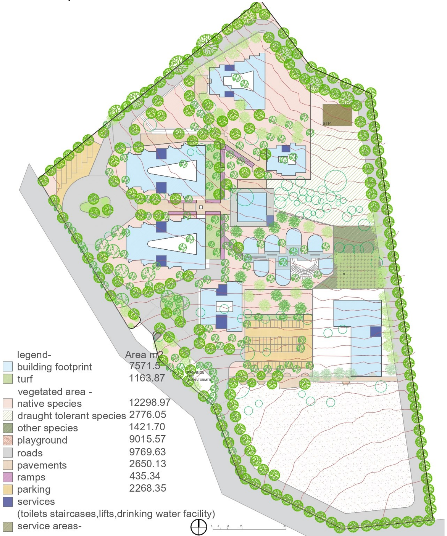
Site plan highlighting Total non-roof area, area covered with trees (foliage) or open grid pavers.
