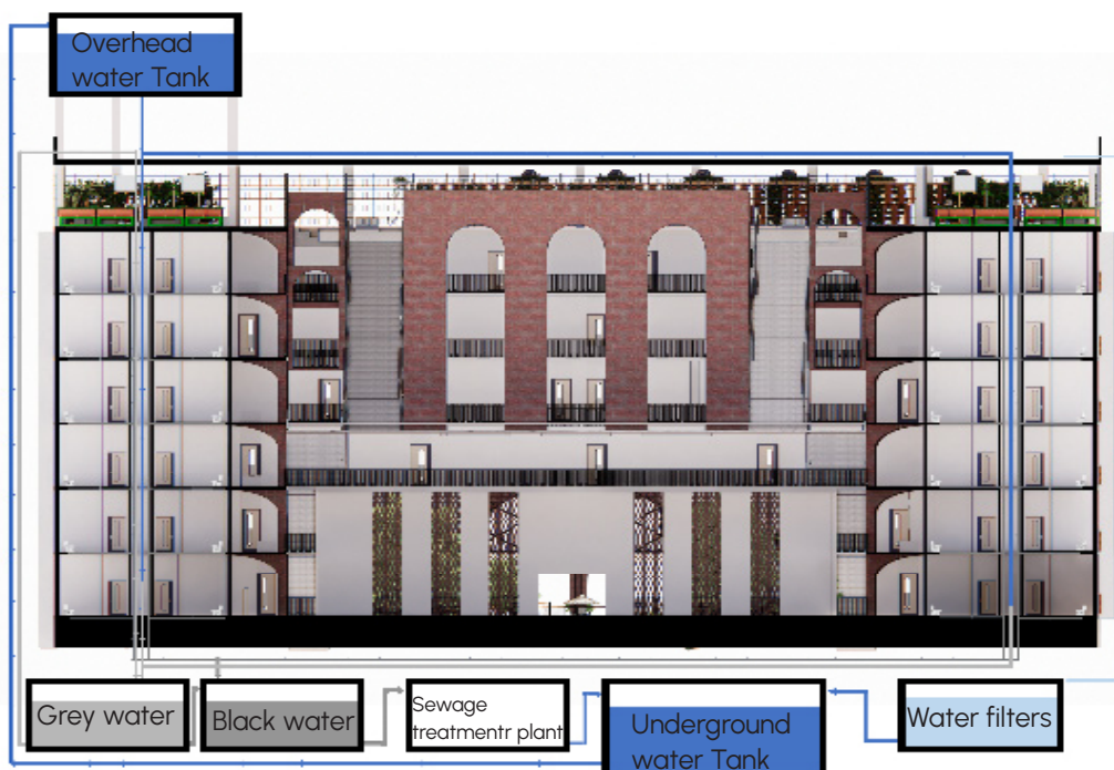
Fig.36 Water treatment system in the design
