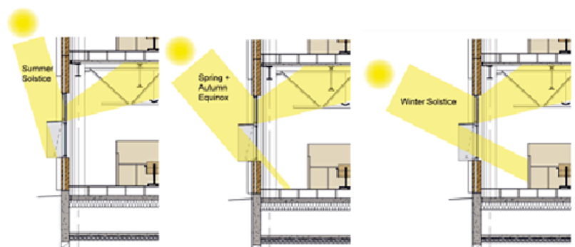
Figure 26: Seasonal performance of shading, redirection devices.
