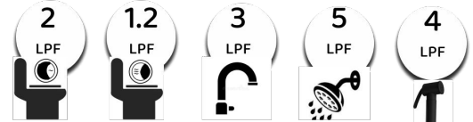
Fig 7.5.1 : Flow Rate Fixtures
