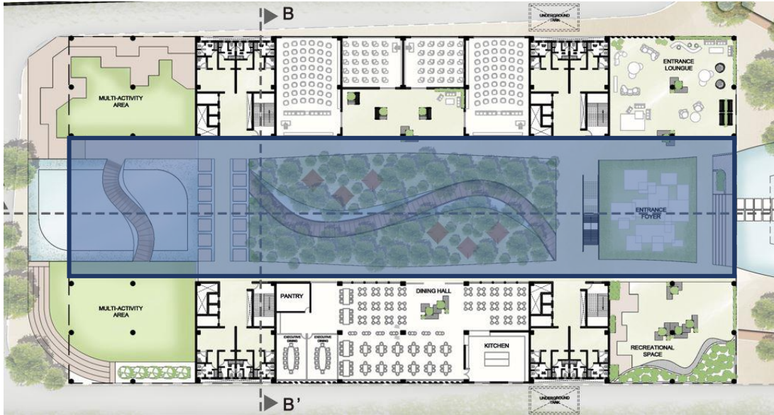
Fig 57 – Plan of the building showing central courtyard roof for BIPV transparent solar panel installation
