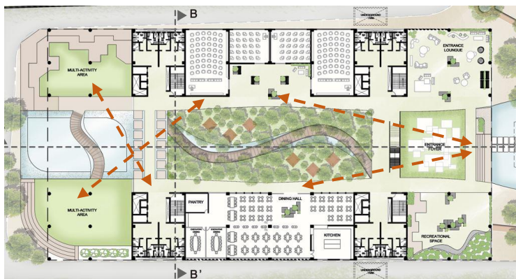
Fig 54– Plan of the building showing horizontal connectivity
