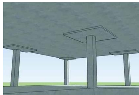
Fig 46 – Flat slab construction
