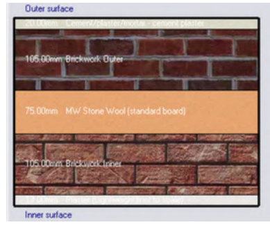
FIG 79. WALL COMPOSITION- BASECASE:
