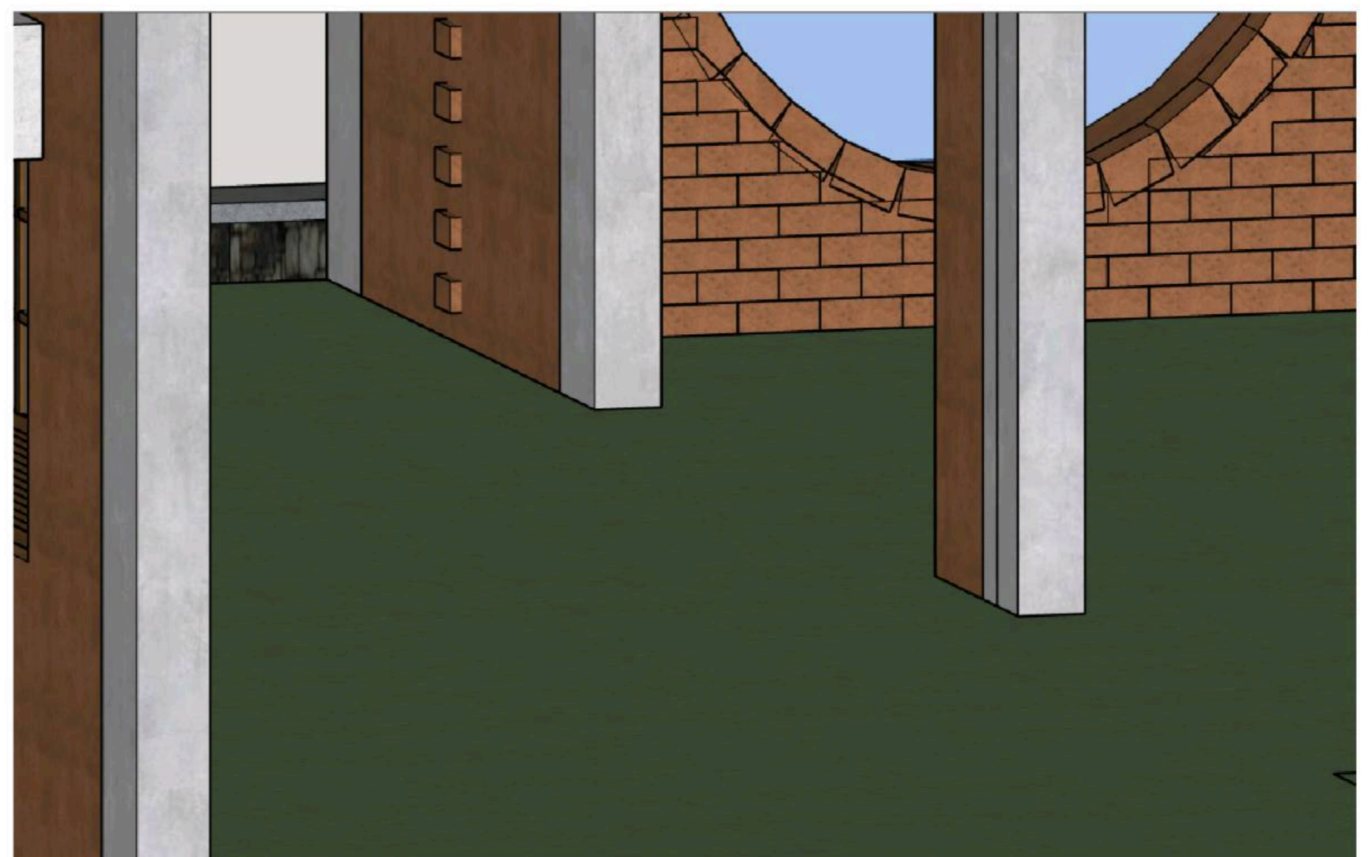
Fig 6.6.4- Green oxide flooring for interior
