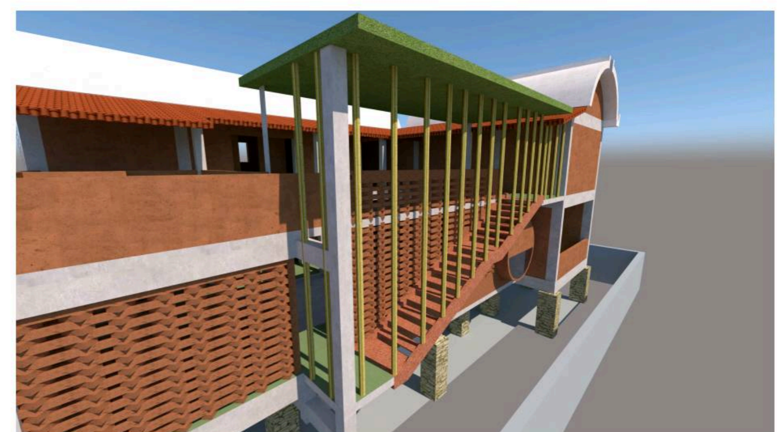
Fig-6.4.11 Barriers for avoiding thermal shock To prevent the thermal shock, numerous barriers have been built. The obstruction is the staircase, followed by the placement of the jali walls.
